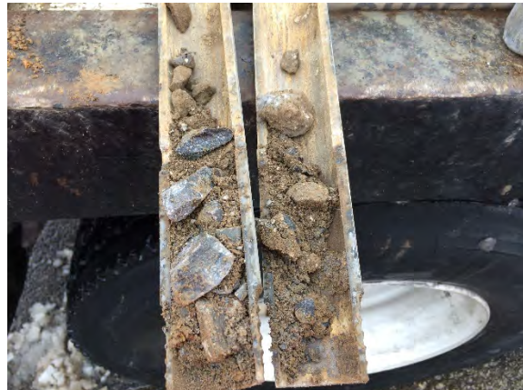
Sample of Fill with broken rock pieces
