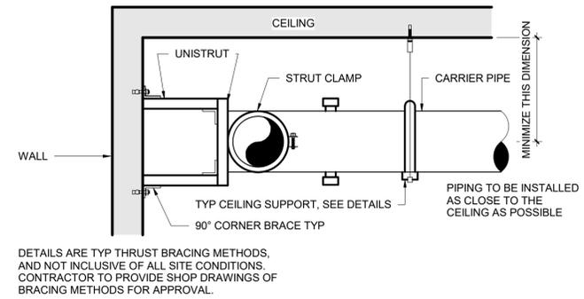
8 | PIPE THRUST BRACING
