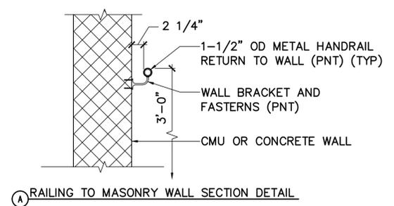
**A RAILING TO MASONRY WALL SECTION DETAIL**
