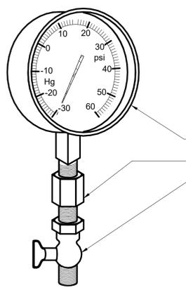
PRESSURE GAUGES SHALL BE INSTALLED BY MEANS OF DRILLING & TAPPING PIPE TO BE MONITORED. THE GAUGE SHALL THEN BE THREADED INTO THE PIPE. PROVIDE WITH SNUBBER & PET COCK.
