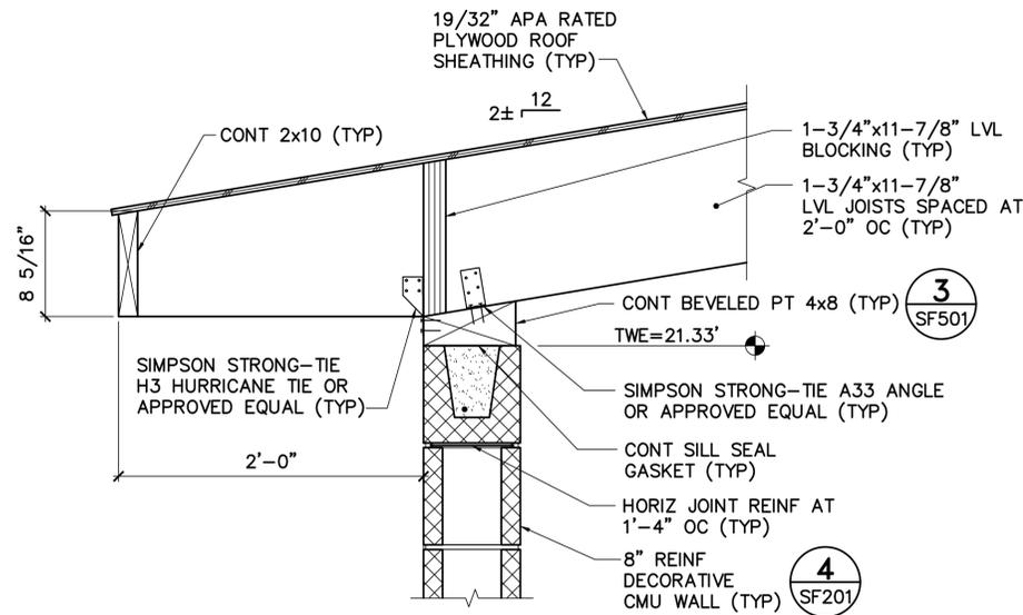
**1** TYP 1-3/4"x11-7/8" LVL JOIST TO 8" REINF CMU WALL CONN DETAIL
