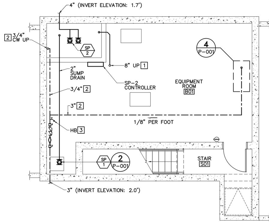
**1 BASEMENT AND UNDERSLAB PLUMBING PLAN**
