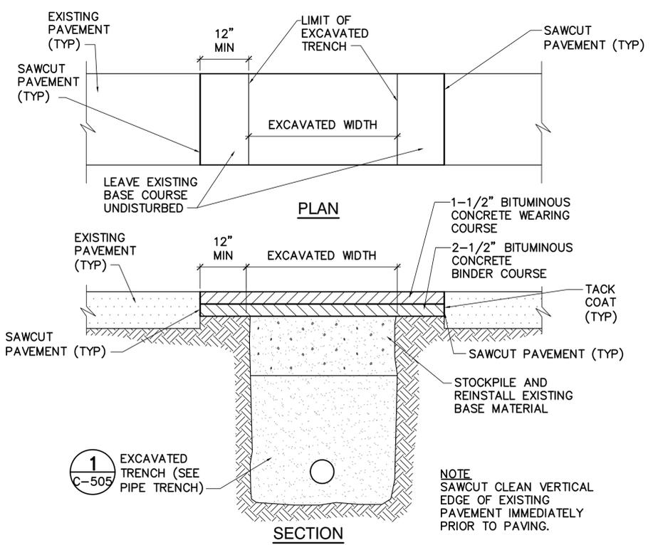
**1 ASPHALT CONCRETE TRENCH REPAIR**
