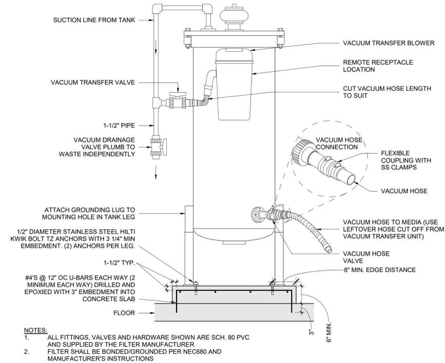
**3** VACUUM TRANSFER SYSTEM AND FILTER PAD DETAIL
