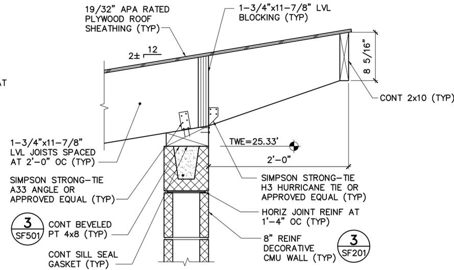
**2** TYP 1-3/4"x11-7/8" LVL JOIST TO 8" REINF CMU WALL CONN DETAIL
