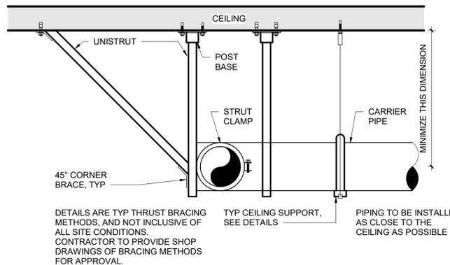
5 | PIPE THRUST BRACING
