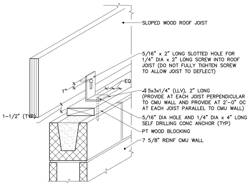
**4 SLOPED JOIST TO CMU INTERIOR WALL**
