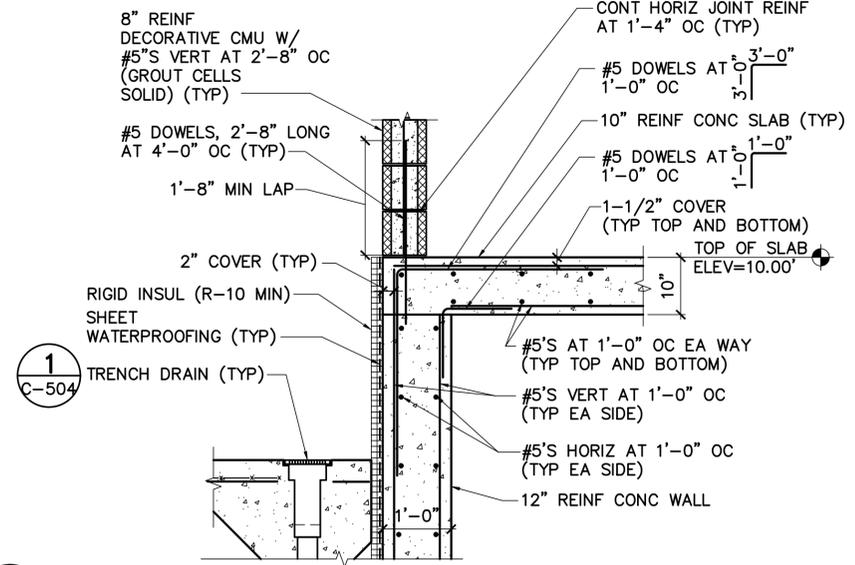
**2 REIN CONC STRUCTURAL SLAB/REIN CONC WALL DETAIL**
