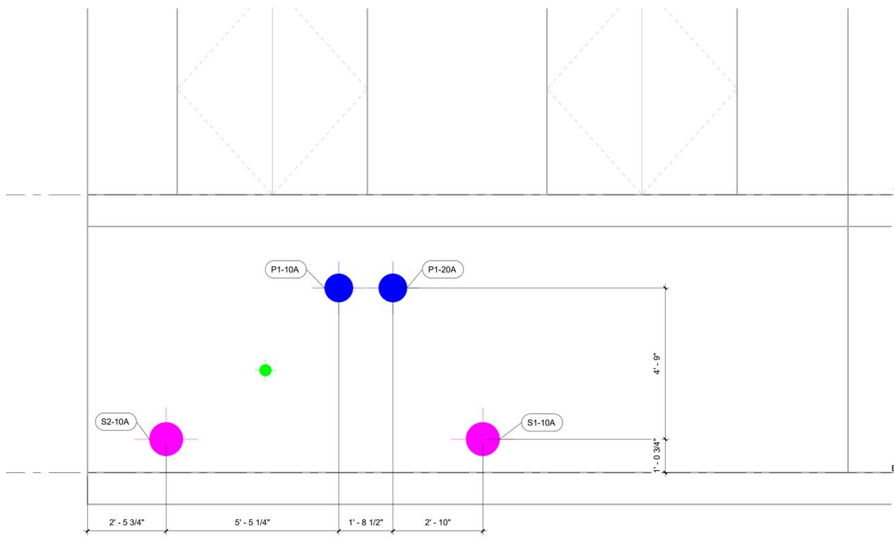
**2** MECHANICAL ROOM PIPE PENETRATION (PLAN SOUTH WALL)
