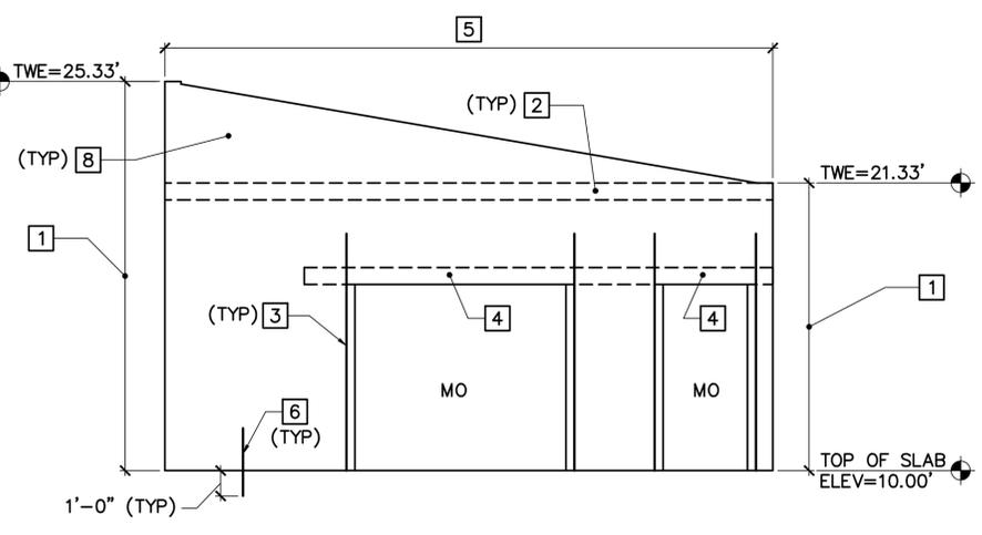
**2 SHEAR WALL 2 ELEVATION (SW2)**
