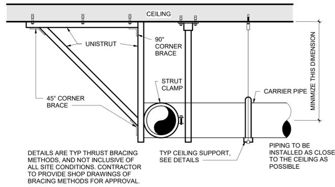
7 | PIPE THRUST BRACING
