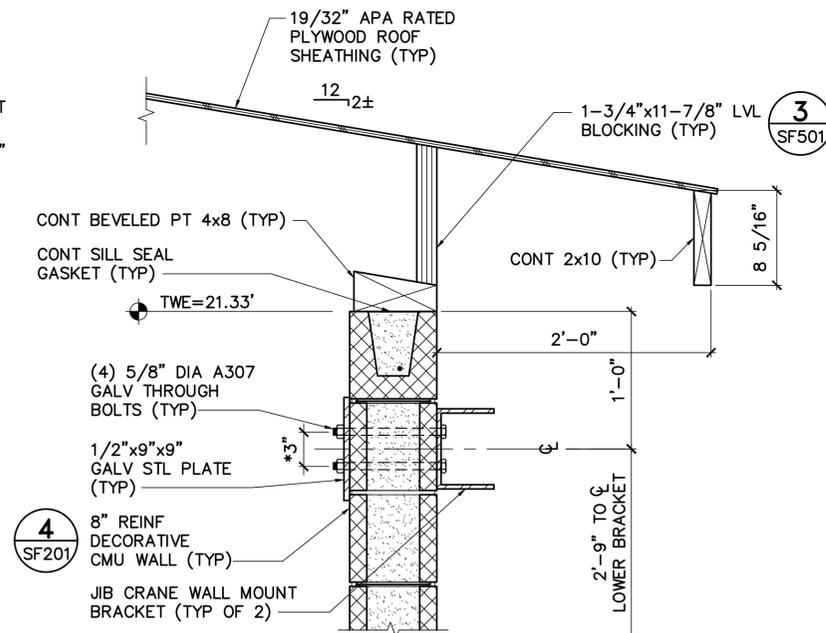
**4** TYP JIB CRANE WALL MOUNT BRACKET CONN DETAIL
