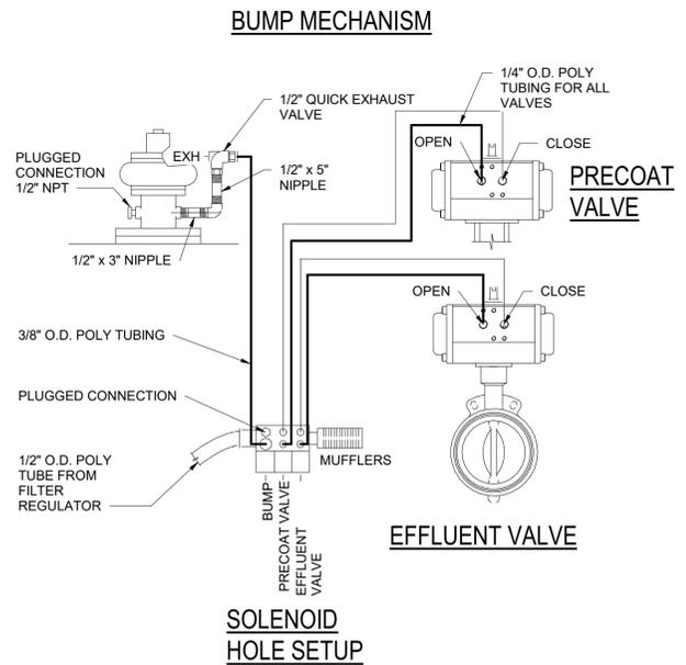
**2** PNEUMATIC VALVE DIAGRAM
