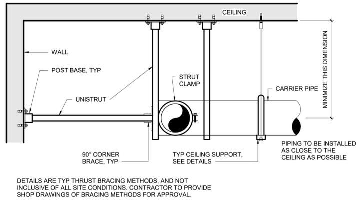
6 | PIPE THRUST BRACING
