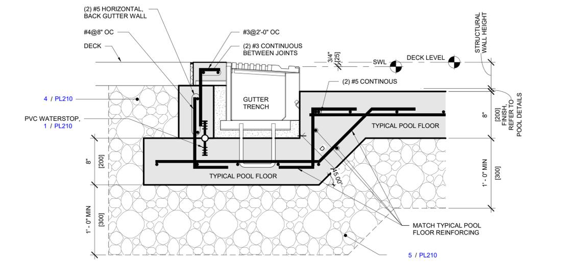
**4** REINFORCING - ZERO DEPTH TRANSITION TO WALL
