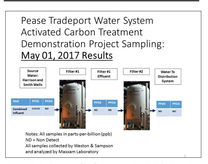
The activated carbon demonstration filters for the Harrison and Smith wells have been on line since mid-September 2016. The City's engineering consultant continues to sample the performance of the filters based on the volume of flow going through the filters. The graphic above shows the most recent source water sampling and treated filter water quality results for the PFOS and PFOA. A summary of all of the sampling and laboratory results is attached.
