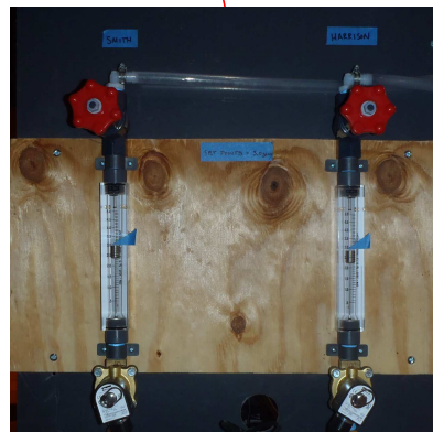
Control flow from wells into tanks
